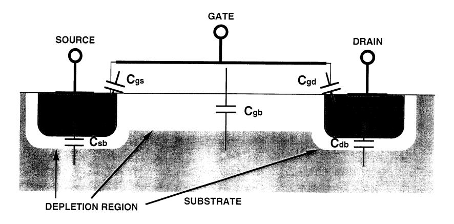
C<sub>sb</sub>, C<sub>db</sub> CAPACITANCE OF REVERSE BIASED p-n JUNCTION (NONLINEAR)
