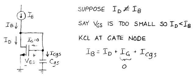
IF ID <IB, THEN ICGS WILL BE POSITIVE THE CHARGING UP CGS TO IB
