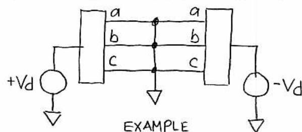
EXAMPLE: by voltage divider,  $V_x = 0$  regardless of  $V_d$ . Therefore we can signal ground this connection without affecting circuit performance
