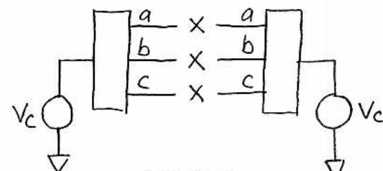
EXAMPLE:  $i=0$  (no voltage drop across  $R_s$  due to symmetrical excitation. We can open this connection without affecting performance)
