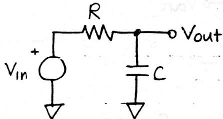
$$\frac{V_{out}}{V_{in}} = H(s) = \frac{1}{1 + sRC} = \frac{1}{1 + s\tau}$$
