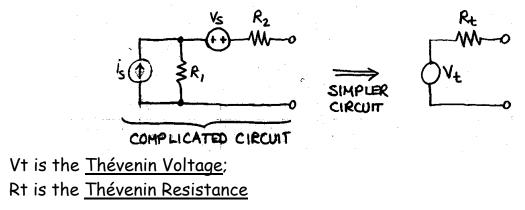
Thevenin's theorem says that, if you choose Vt and Rt correctly, the simple circuit of one source and one resistor will have the exact same V-I characteristic as the more complicated circuit. How do you choose Vt and Rt correctly? Usually the simplest way is to use the following procedure to find:
