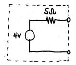
Now we can hook Rx back up, and the resulting circuit is easier to work with.
