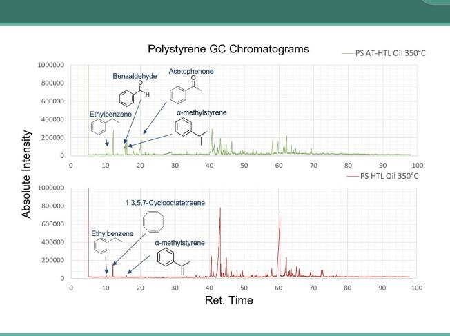
Figure 1 (left) is a GC chromatogram of polystyrene HTL with and without H<sub>2</sub>O<sub>2</sub>. Data courtesy of Dr. Timko's team and Elizabeth Belden at Goddard Labs at WPI. Figure 2 (right) is a calibration curve of styrene created by Elizabeth Belden. Different concentrations of styrene were placed in GC-MS, creating an equation.
