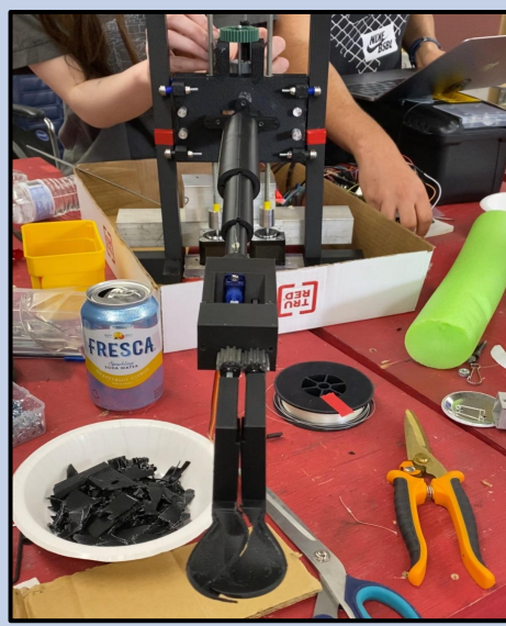
Figure 9: Set up of experiment, motor was being replaced.
