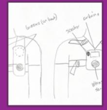
Design #3 Pros: Modular, adjustable Cons: Bulky, long hair interferes with function, sensors on the back
