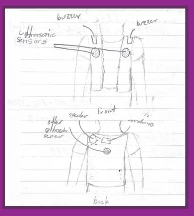
Design #2 Pros: Simple to use Cons: Difficult to attach sensors, wires on both sides, sensors on the back
