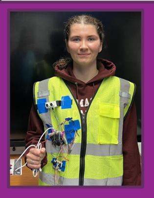
Pros: Detects flat objects such as walls, reasonably easy to put on, low-cost, modular design Cons: Does not detect smaller objects, varying results with small changes in angle, fragile due to use of non-preferred materials, connected to laptop, vibration motor does not work
