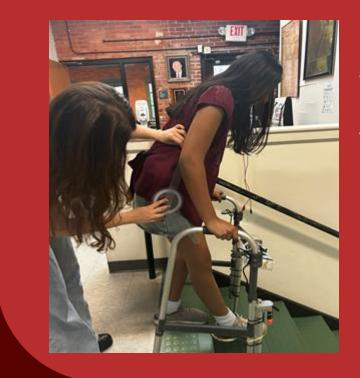
**Purpose:** To determine which prototype design (control/no walker, walker with button, and walker with ultrasonic distance sensor) allows for the least possible movement. Independent Variable: Main prototype designs Dependent Variable: Angle at two pivots: hip and knee **Procedure:** The angles will be measured using a goniometer placed at two joints.
