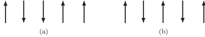
Figure 5.19: Microstates corresponding to two flipped spins of a system of N = 5 spins in one dimension. In (a) the flipped spins are nearest neighbors and in (b) the flipped spins are not nearest neighbors.
