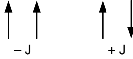
Figure 5.1: Two nearest neighbor spins (in any dimension) have an interaction energy -J if they are parallel and interaction energy +J if they are antiparallel.
