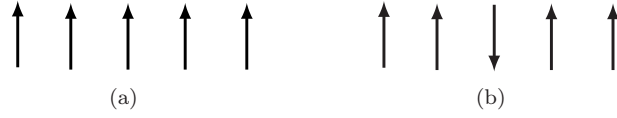
Figure 5.18: (a) The ground state of N = 5 Ising spins in an external magnetic field H . For toroidal boundary conditions, the ground state energy is E_0 = -5J - 5H . (b) The flip of a single spin of N = 5 Ising spins. The corresponding energy cost is 4J + 2H .
