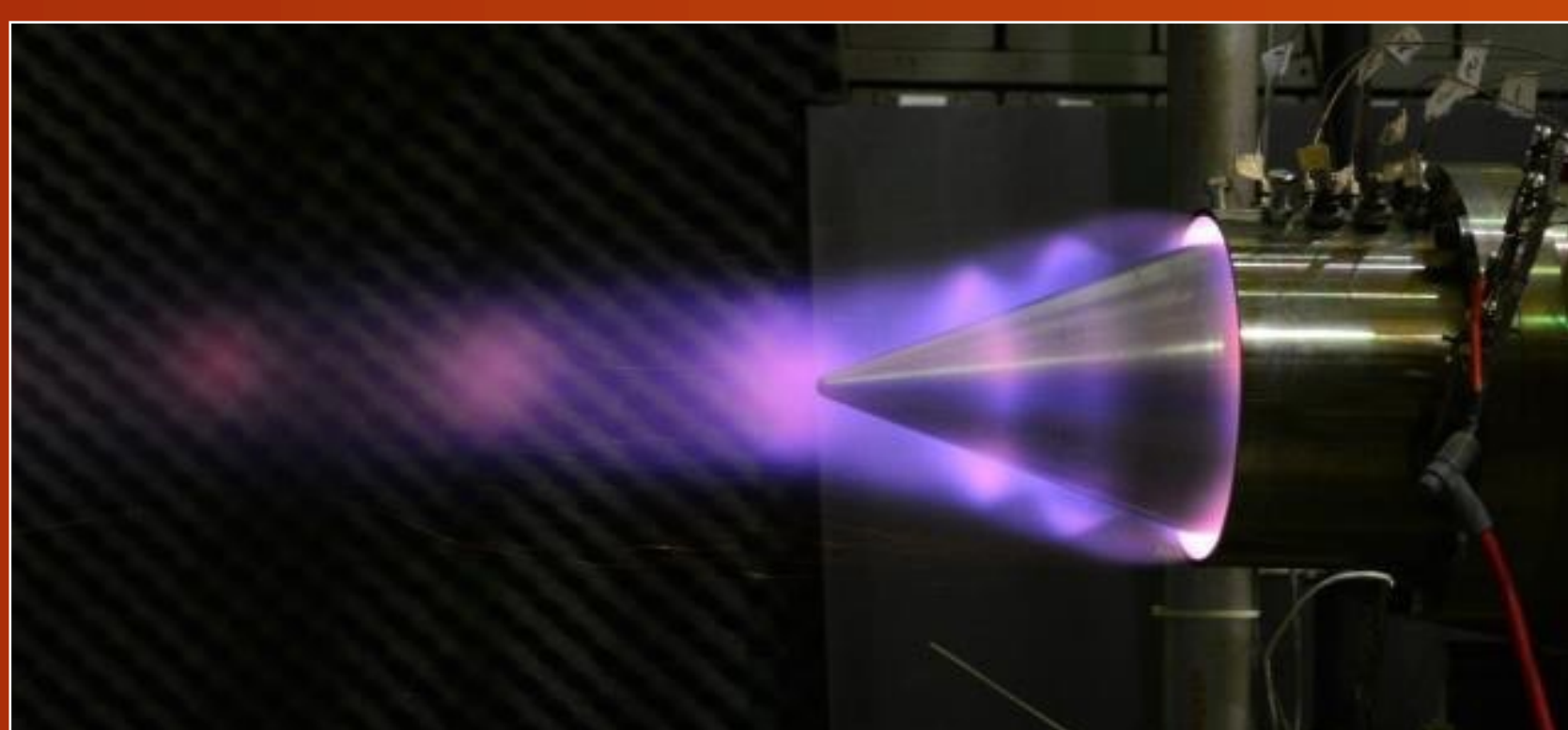
The Rotating Detonation Engine: Experimental RDE from the Air Force Research Laboratory.
