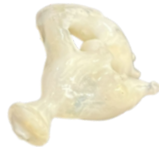
Figure 3: Shell cast 3D-printed with a resin printer and filled with silicone.
