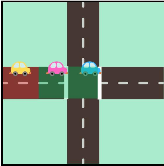
For instance, in the diagram, the yellow car would stop since it can stop before the white line, while the pink and blue cars must go. The red represents the stop zone while the green represents the go zone.
