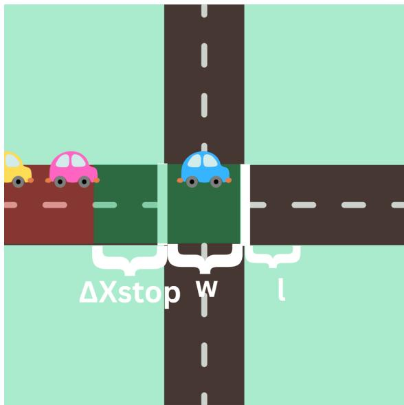
For instance, the pink car does not have enough distance to stop, so it must cross the intersection. Thus, the yellow light must last long enough for the pink car to cross the minimum distance to stop, the width of the intersection, and the length of itself.
