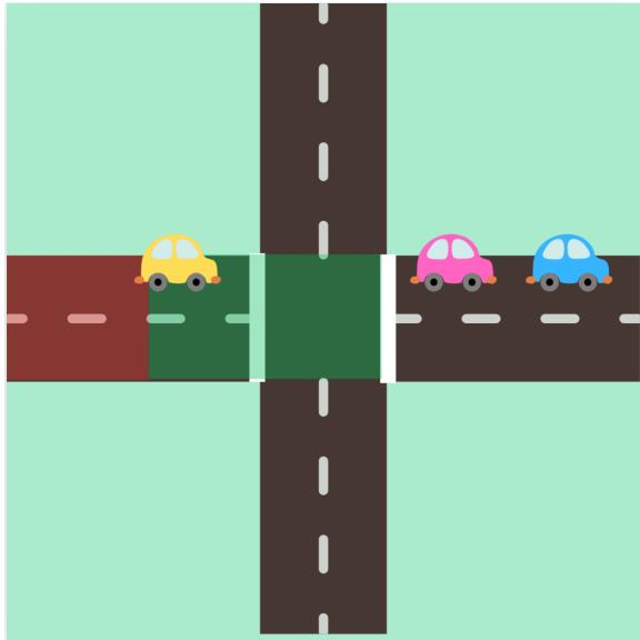
In this scenario, the light has turned red. The pink and blue cars have fully crossed and are safe. Notice that the yellow car has not reached the white line even though the light is red, yet it is still not dangerous. Thus, the yellow light time is not dependent on the time it takes to stop the car.
