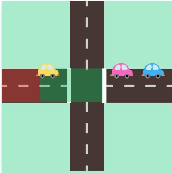
In this scenario, the light has turned red. The pink and blue cars have fully crossed and are safe. Notice that the yellow car has not reached the white line even though the light is red, yet it is still not dangerous. Thus, the yellow light time is not dependent on the time it takes to stop the car, and is instead dependent on the longest amount of time needed for a car to fully and safely cross the intersection. We began looking into how to find this.
