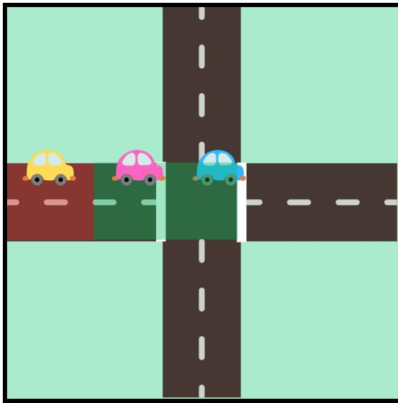
For instance, in the diagram, the yellow car would stop since it can stop before the white line, while the pink and blue cars must go. The red represents the stop zone while the green represents the go zone. We started basing our ideas to solve the problem off of this.
