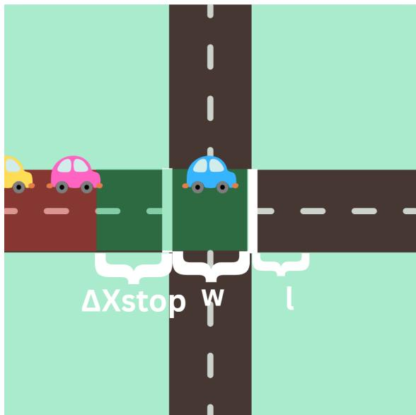
For instance, the pink car does not have enough distance to stop, so it must cross the intersection. Thus, the yellow light must last long enough for the pink car to cross the minimum distance to stop, the width of the intersection, and the length of itself, since the back of the car needs to fully get across the intersection too.
