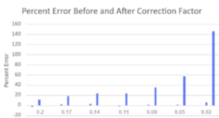
Figure 6. Percent error of pump before and after adjusting for constant correction factor.
