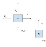
The free body diagram in Figure 2 shows the forces acting on the masses in the modified Atwood's machine. This free body diagram allowed us to derive the equations found below. We decided that positive motion is to the right for the cart, and down for the hanging mass.
