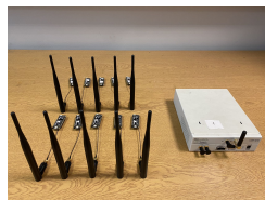
Fig. 5. LoRa transmitters and a USRP receiver.
