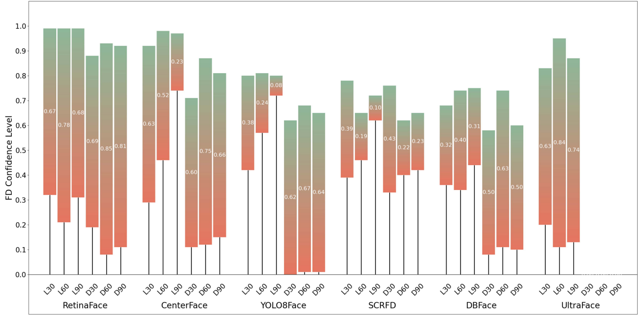
Fig. 10. Confidence reduction across different FD models due to EoA adversarial attack.
