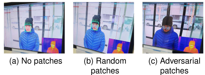
Fig. 8. Attacking the commercial surveillance camera.
