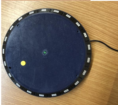
Figure 2: Bird's eye view of the Roulette design with both pieces connected. The wire inserted into the device from the right side provides power to the arduino and stepper motor. The LED positioned at the center of the device functions as a reminder system, blinking when the time is right to take medication. The yellow button at the lower left end side of the device will stop the LED from blinking once the user takes the medication.
