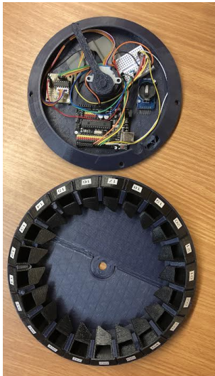
Figure 1: Bird's eye view of the Roulette design. The top half of the image is the lid of the device. Included within the lid are an arduino UNO, a stepper motor, its driver, and a "pushing" rod. The bottom half of the image is the container of the device. The device includes 21 slidable compartments, labeled 01 - 21, 01 standing for Monday morning, and 21 standing for Sunday evening. 02 would therefore equate to Monday afternoon, and so on for one full week. The compartments are capable of holding 14 pills.
