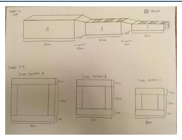
Planned wind tunnel made out of polyfoam and plexiglass. The hatches are where one can put the models into the wind tunnel.
