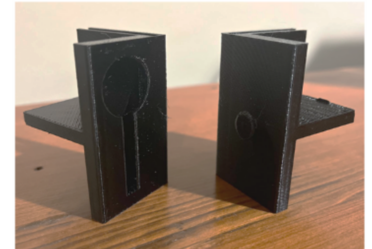
Design 4: Locking slider mechanism
