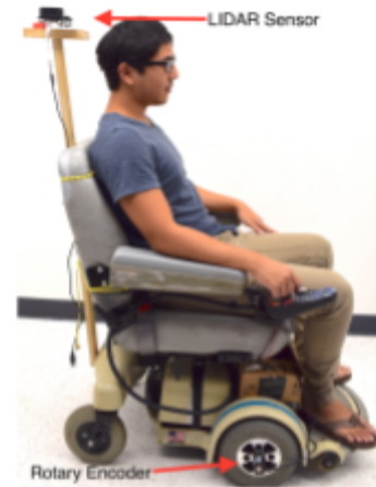
Figure 7. Wheelchair affixed with LiDAR sensor and rotary encoders.
