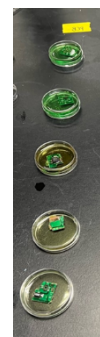
Figure 3. Impact of nitric acid concentration on EC removal. From top to bottom: 40%, 35%, 30%, 25% and 20%.
