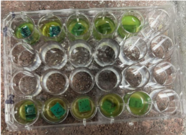
Figure 6: Tests to compare 1M and 2M KOH at different S/L ratios. Group 1 (top row) is 1M KOH. Group 2 (bottom row) is 2M KOH. From left to right are S/L ratios: 1g:1ml, 1g:2ml, 1g:3ml, 1g:4ml, 1g:5ml, respectively.
