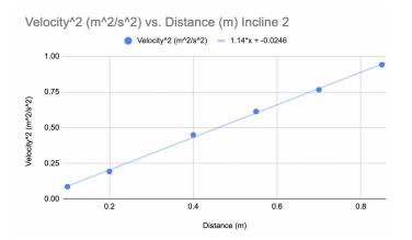
The equation,  $V_f^2 = V_0^2 + 2a\Delta x$ , can be linearized so that  $V_f^2$  is y,  $\Delta x$  is x and the slope is 2a.  $V_0^2$  is the y-intercept but can be disregarded because  $V_0$  is always 0 m/s.
