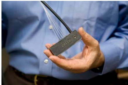
Figure 2. One fNIRS probe. In a typical setup, two probes placed on the forehead. The thin clear fibers are attached to the LEDs and the black, thicker fiber is attached to the light detector. A headband holds the probes in place.
