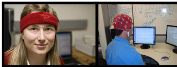
Figure 1. fNIRS (left) and EEG (right) provide useful cognitive and affective state information while remaining non-invasive and practical for HCI settings.
