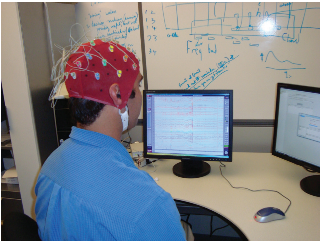
Figure 6.1: Electroencephalography (EEG) measures electrical activity originating in the cortex through electrodes placed on the scalp.
