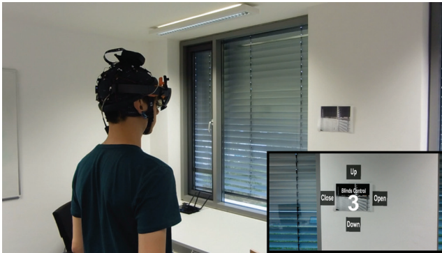
Figure 9.1: Smart room control based on Augmented Reality using brain input (Putze et al. , 2019).
