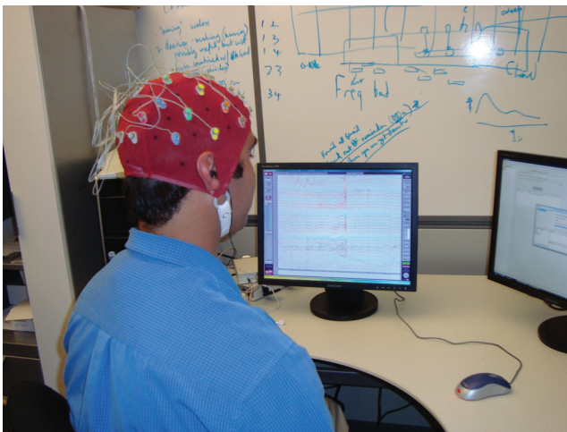
Figure 6.1: Electroencephalography (EEG) measures electrical activity originating in the cortex through electrodes placed on the scalp.
