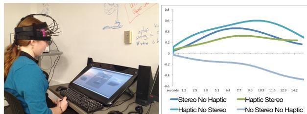
Figure 1. Left: zSpace 3D stereoscopic display and fNIRS brain sensors. Right: Average change in oxy-hemoglobin in Level 5.
