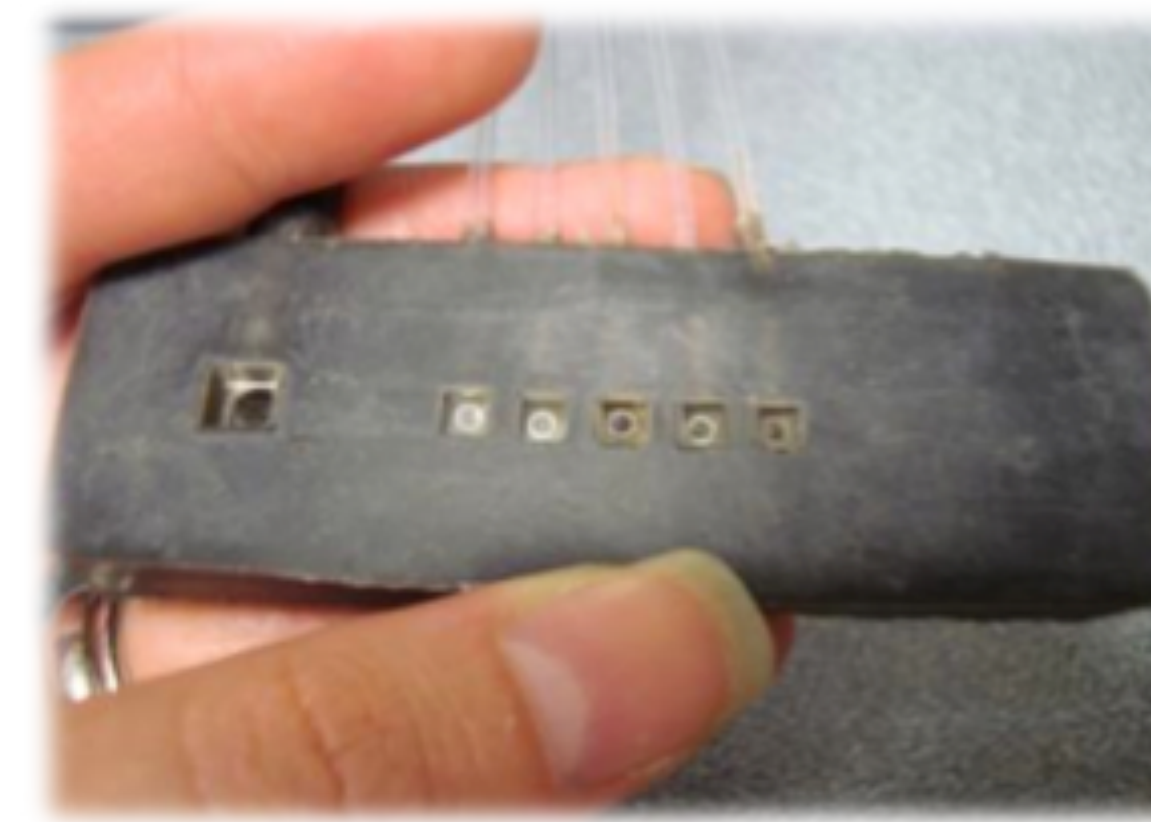
Fig 2. OxiplexTS (ISS Inc.) Each source emits two light wavelengths (690/830nm) to detect both oxygenated and deoxygenated hemoglobin. Source - detector distances were 1.5, 2, 2.5, and 3cm
