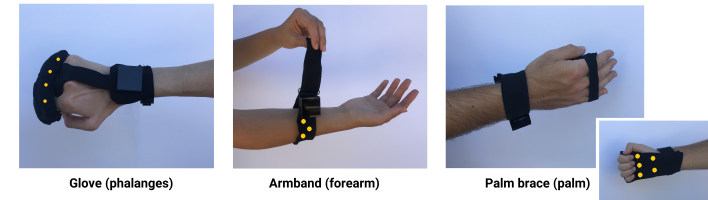
Figure 1: Three stimulation devices used in the study. Each device contains 5 actuators of each type. Locations of the actuators are indicated by yellow dots; not all actuators are visible.
