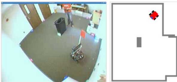
Figure 11. The Brain-Adaptive Human-Robot Interaction Platform supports robot navigation (real or simulated), as well as fNIRS cognitive state input (real or simulated).
