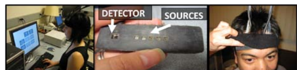
Figure 1. Functional near-infrared spectroscopy is a portable non-invasive tool for detecting brain activity.
