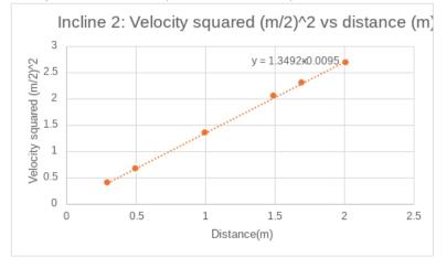
Next, it is time to find the experimental accelerations. To do so, we used the slope of the line of best provided by each of the graphs. The slope of the two graphs is equal to 2a (the m value of our linearized equation). Here was the work conducted to find the experimental accelerations.
