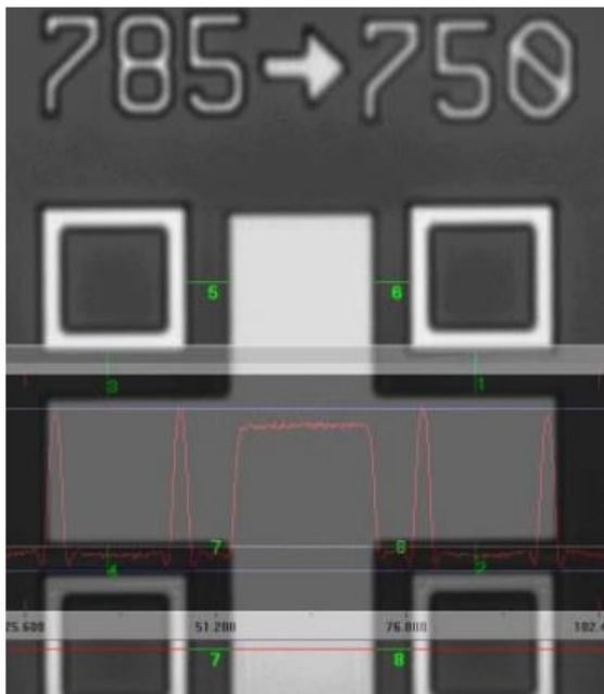
Figure 2a . Combined alignment fiducial measurements by IR metrology system enabling overlay calculations
