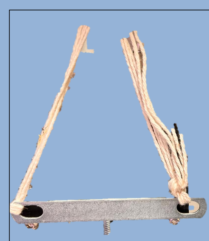
Image 4: Image of the apparatus used to replace the u-bolt for nests that were unable to have the u-bolt wrapped around it. This apparatus consists of a string looped over multiple times and the top part of a U-bolt.
