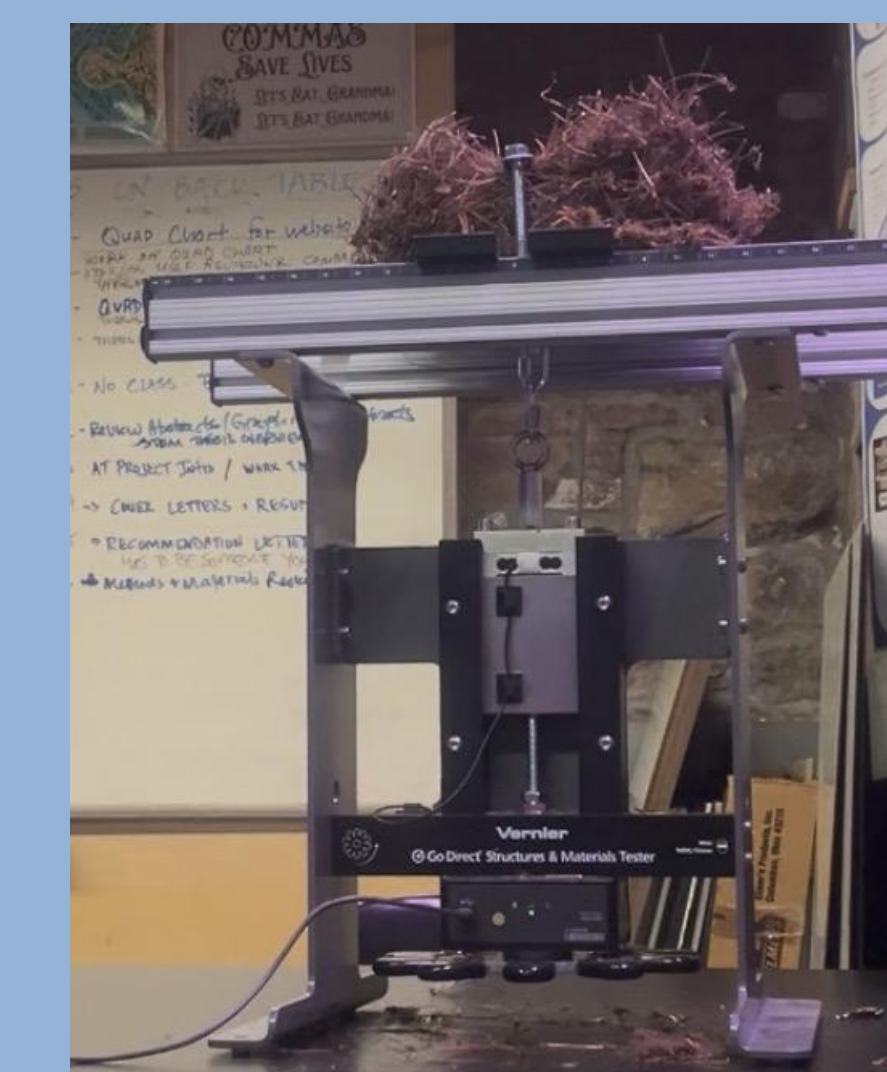
Image 4: Image of the Vernier Structure and Materials tester. The nest was on the top, and the U-bolt was wrapped around the nest.
