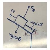
We began by creating a Free-Body Diagram to identify all the forces acting upon the puck. By doing that, we were able to find out that there are four total forces acting on the puck: the normal force, the two components of gravity, and the force of friction (shown in diagram). Using all those forces, we were able to come up with a derived equation for the forces acting on the puck:
