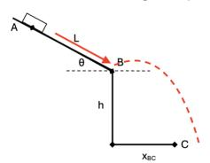
until the ramp suddenly reaches a vertical drop, from where the puck becomes a projectile (refer to the figure to the right). We were tasked with finding out how far the puck lands away from the from the base of the counter. Then, we were tasked with finding a way to change the angle of the ramp's incline to maximize the distance that the puck travels (as a projectile).
