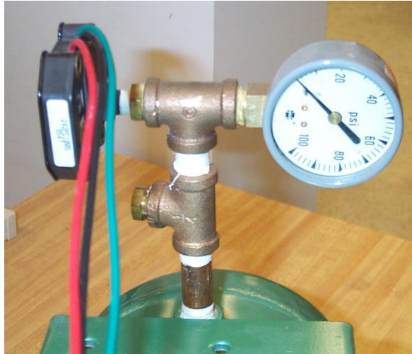
Figure 4: Enlarged view of pressure gage and pressure transducer with its 3 wires (red, black, and blue)
