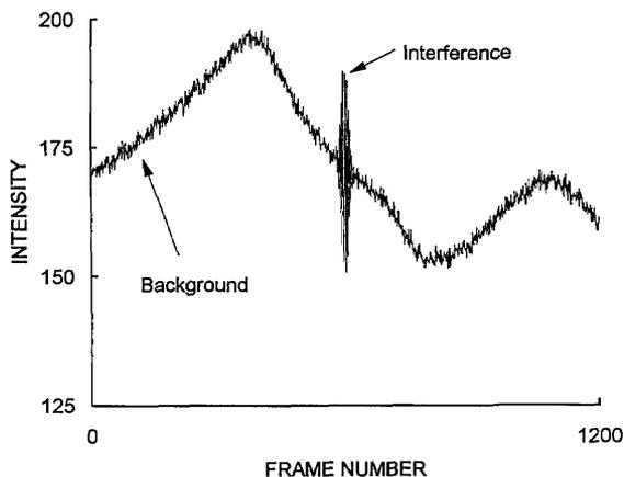
Fig. 2. Intensity history from a single pixel during a 100- $\mu\text{m}$  scan when a broadband source is used. The intensity, digitized to 8-bit precision, versus the camera frame number is plotted during the scan.
