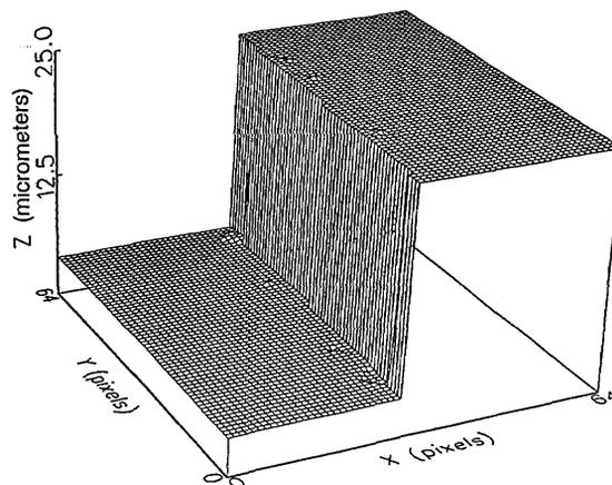
Fig. 5. Measurement of a  $20.37\text{-}\mu\text{m}$  step-height standard measured with the SWLI profiler.
