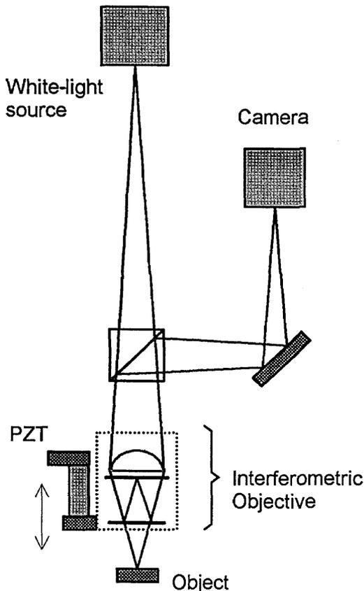
Fig. 1. Schematic diagram of the SWLI profiler. PZT, piezoelectric transducer.
