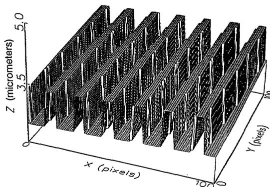
Fig. 6. Measurement of a 921-nm-high grating with the SWLI profiler.
