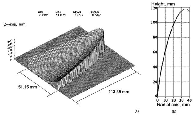
**Fig. 9** Measurement of absolute shape: (a) 3-D wire-frame representation obtained by sampling Fig. 8(b) every 6 pixels, (b) measured data points and curve fitting results corresponding to the meridian curve of the paraboloid-of-revolution section. The meridian is defined by a parabolic equation of the form  $y = 0.1097x^2$  [mm], obtained with a confidence interval near  $10 \mu\text{m}$ .
