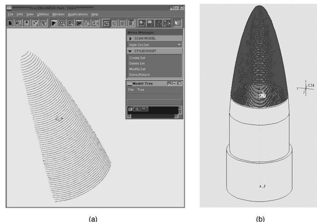
**Fig. 10** Measurement of absolute shape: subsampled  $(x,y,z)$  data clouds of measured sections imported into a CAD environment (Pro/Engineer); (a) single section and (b) tiled sections used for defining the geometry of the entire component.
