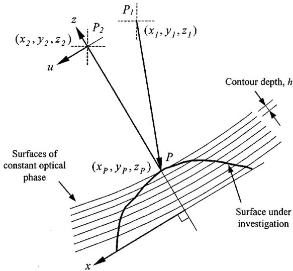
**Fig. 5** Geometrical representation of the two-wavelength optical setup used in the determination of surface shape.  $P_1$  is the point of illumination,  $P_2$  is the point of observation,  $P$  is a point on the surface under investigation, and the plane  $(x,y)$  is parallel to the image plane  $(u,v)$ .
