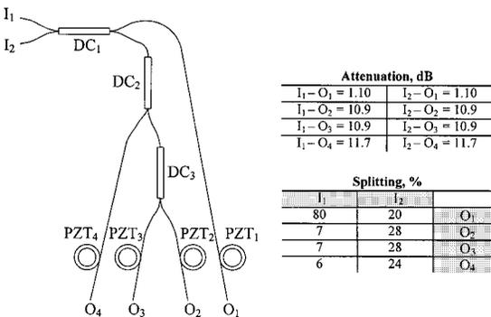
**Fig. 2** Single-mode fiber-optic-based directional coupler assembly (FA in Fig. 1): I<sub>1</sub>, I<sub>2</sub> are the FC-connectorized input fibers, DC<sub>1</sub>, DC<sub>2</sub>, and DC<sub>3</sub> are the directional couplers, PZT<sub>1</sub>, PZT<sub>2</sub>, PZT<sub>3</sub>, and PZT<sub>4</sub> are the ceramic piezoelectric cylinders, and O<sub>1</sub>, O<sub>2</sub>, O<sub>3</sub>, and O<sub>4</sub> are the FC-connectorized output fibers.
