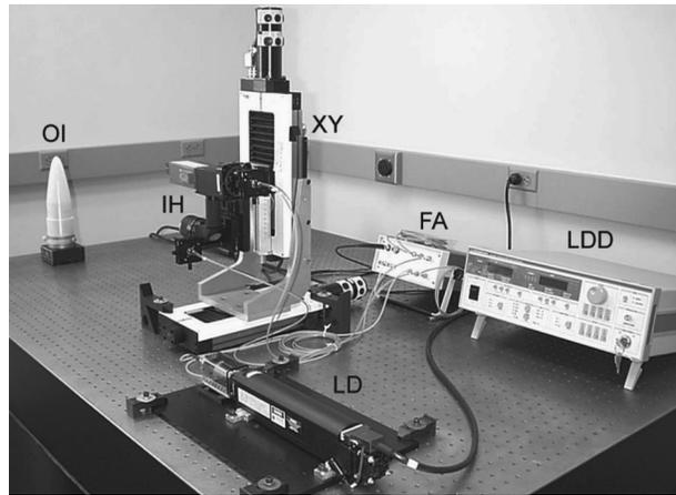
**Fig. 3** Fiber-optic-based OEH setup arranged to perform high-resolution surface shape measurements: LD is the laser diode, LDD is the laser diode driver, FA is the single-mode fiber optic directional coupler assembly, XY is the X-Y translational stage, IH is the interferometric head, and OI is the object under investigation.
