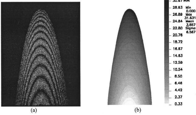
**Fig. 8** Measurement of absolute shape: (a) one of the six OEH interferograms obtained at 60-deg increments of the rotational stage, (b) corresponding analysis showing 106,269 pixels with shape information. Camera range  $940 \pm 3$  mm, providing a spatial resolution of  $0.1975$  mm/pixel and a contour depth uncertainty near  $10 \mu\text{m}$ .
