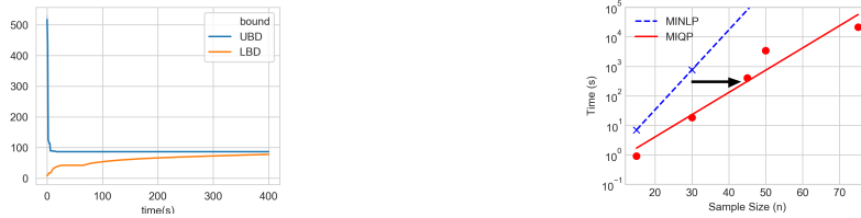
(a) Convergence of upper and lower bounds for MIQP method. (b) MIQP improves upon the MINLP solution computation time as shown by the shift of curve to the right.
