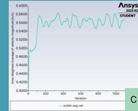
Plot of Area-Weighted Average of fan velocity over iterations.
