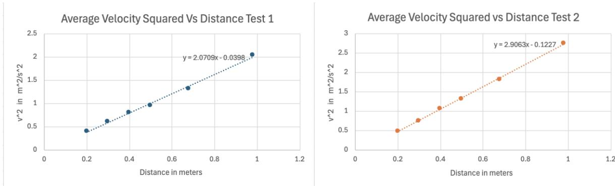
Test 1 is an experiment where 3 books (incline 1) were used while test 2 is the experiment where 4 books were used (incline 2).
