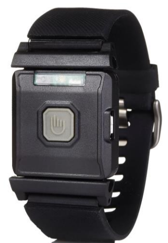
Figure 10: TouchPoint Wristband. Tracks heartbeat and other physical identifiers to identify an episode.
