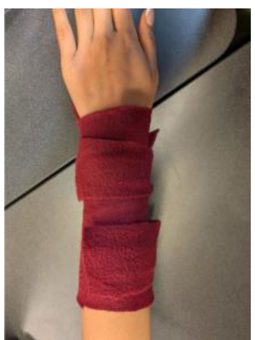
Figure 1: Vibration Sleeve Design. Cons: The fabric was bulky and caused sweating.
