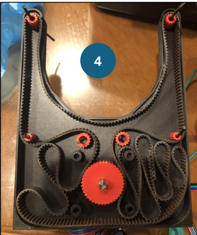
Figure 8a & 8b: Retainer case + timing track + gears in two iterations – we finalized the second design (5)
