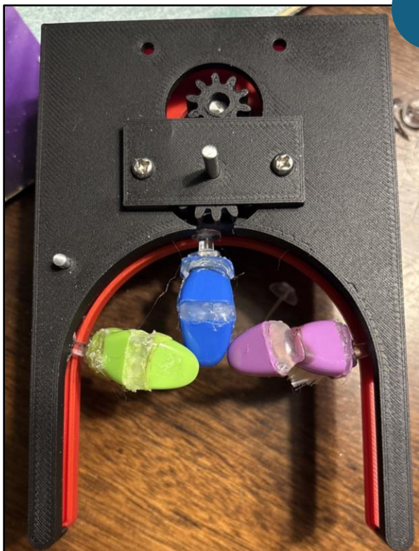
Figure 8a & 8b: Retainer case + timing track + gears in two iterations – we finalized the second design (5)
