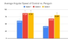
Figure 1: Average Angular Velocity (AV) of the Standard Wind Turbine Blade and Penguin Wing over 3 Wind Speeds. The Control had an average angular velocity of 87.8 rad/s for wind speed 1, 87.8 rad/s for wind speed 2, and 87.8 rad/s for wind speed 3. The penguin wing design had an average angular velocity of 62.5 rad/s for wind speed 1, 68.8 rad/s for wind speed 2, and 80.9 rad/s for wind speed 3. Overall, the control was faster, however, reached its optimal wind speed at wind speed 2, only seeing a minor improvement for wind speed 3. The penguin wing design was on average slower, however more consistent, and had a greater amount of improvement for each wind speed compared to the control.
