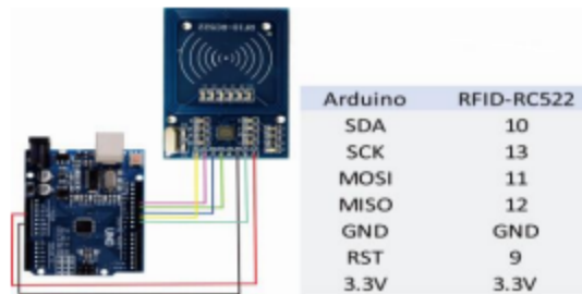
RFID connection with Arduino with what ports they connected each element to
