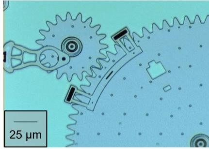
Close-up of the gears of a  $\mu$ -engine
