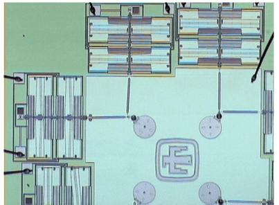
Electrostatically driven  $\mu$ -engines
