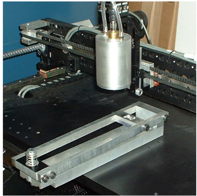
Fig. 4 Photograph of the welding fixture mounted to the welding table. A description of the fixture based on the lower figure: the arms pivot at the far right of the photograph. The “absorbing” part is placed in a slot approximately 2 in. from the pivot and the “transparent” part is placed on top of this part in a T-joint. This “transparent” part is held in place by a rotating carriage, which is the second pivot on the pair of arms. On the far left side of the arms, a precision spring is used to apply pressure. By compressing the spring a specified amount, a known load is applied, allowing the clamping pressure in the weld zone to also be known.
