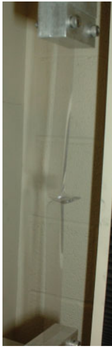
FIG. 4. A sample mounted in a T -peel arrangement in the custom grips. This test is designed to measure the force required to peel apart the spot welded samples. [Color figure can be viewed in the online issue, which is available at www.interscience.wiley.com .]
