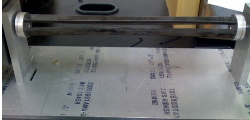
Figure 7. Manufactured torsion spring
